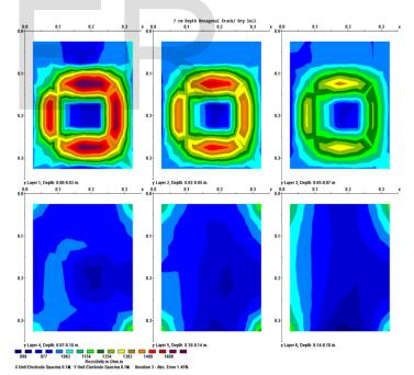
Fig. 3. The inverted resistivity sections of the 7 cm- depth hexagonal crack in dry soil
