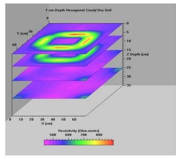
Fig. 4. 3D visualization of the7cm- depth hexagonal crack model in dry soil
