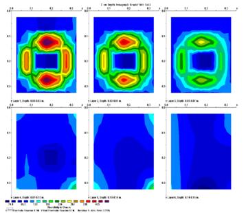
Fig. 6. The inverted resistivity sections of the 7 cm- depth hexagonal crack in wet soil
