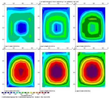
Fig. 12. The inverted resistivity sections of the 7 cm- depth hexagonal crack in wet soil covered by 5cm thickness sediments
