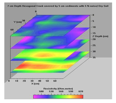
Fig. 11. 3D visualization of the 7cm- depth hexagonal crack with 5% noise in dry soil covered by 5cm thickness sediments
