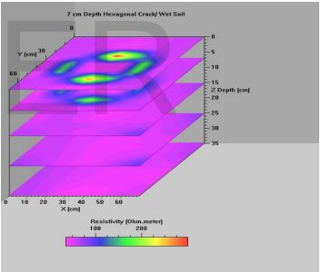
Fig. 7. 3D visualization of the7cm- depth hexagonal crack model in wet soil
