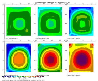
Fig. 9. The inverted resistivity sections of the 7 cm- depth hexagonal crack in dry soil covered by 5cm thickness sediments
