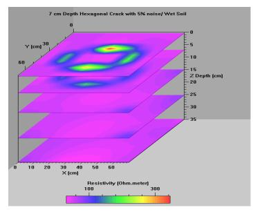
Fig. 8. 3D visualization of the 7cm- depth hexagonal crack with 5% noise in wet soil
