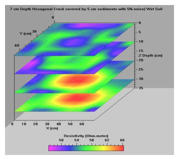
Fig. 14. 3D visualization of the 7cm- depth hexagonal crack with 5% noise in wet soil covered by 5cm thickness sediments
